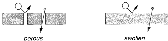
Figure 1.4: Schematic drawing of separation of uncharged molecules by nanofiltration membranes. At the left-hand side a porous membrane and at the right-hand side a membrane with a network swollen structure
